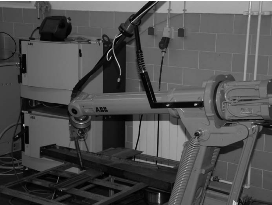
Figure 4.11. Experimental setup used for the TCP/IP sockets server example (ABB IRB1400 robot + ABB IRC5 robot controller)
